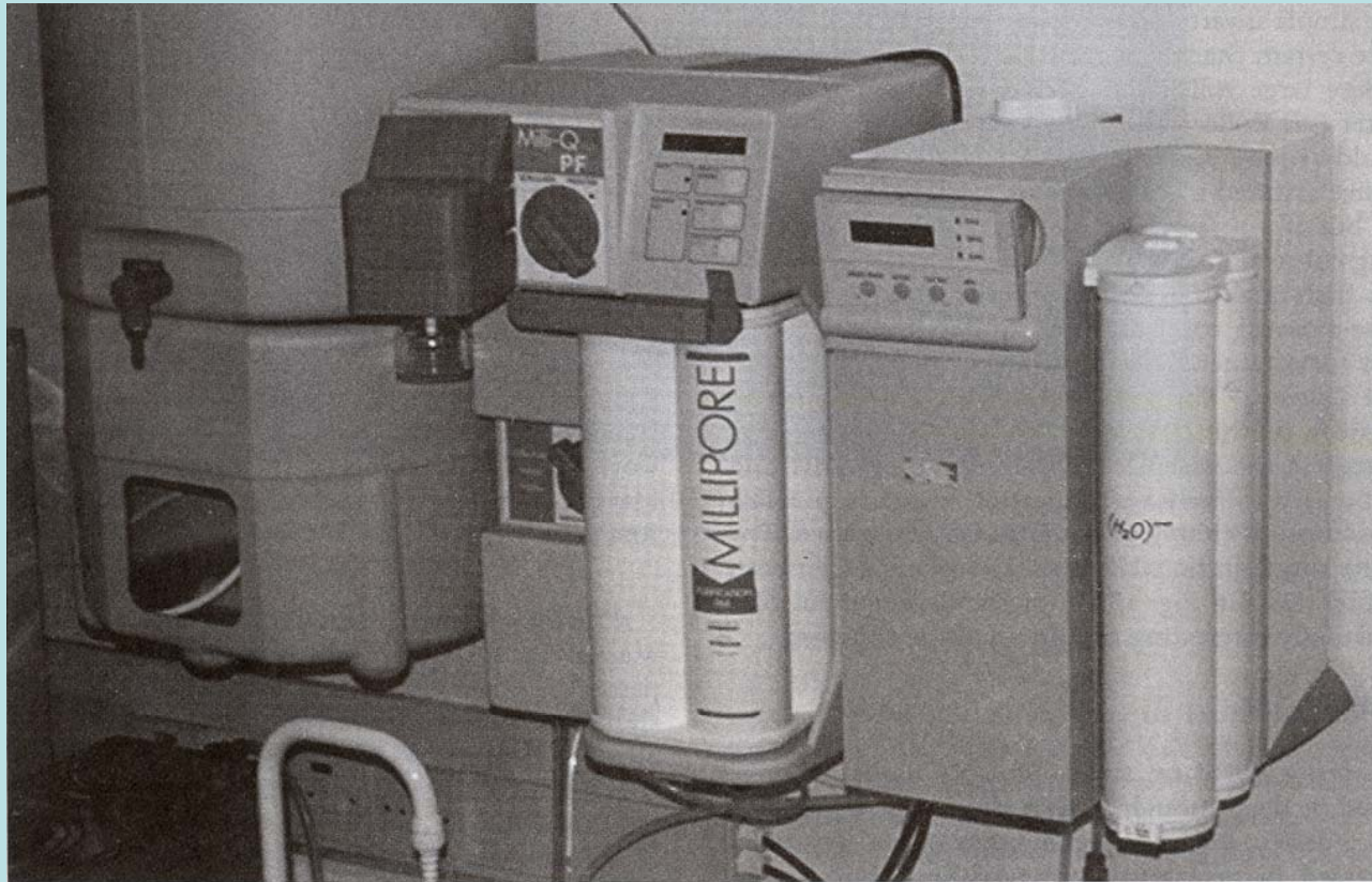
Fig. 4.7. Preparation of Ultrapure Water. Tap water first passes through a reverse-osmosis unit on the right and then goes to the storage tank on the left. It then passes through carbon filtration and deionization (center unit) before being collected via a micropore filter (Millipore MillQ).
